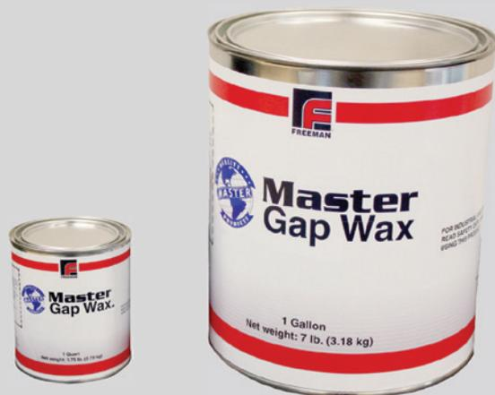
Master Gap Wax is a soft wax developed for quickly and easily filling gaps in sheet wax as well as patching, fixturing and filleting. Master Gap Wax is applied at room temperature and can be used as an alternative to clay, especially when adhesion to the composite material is preferred.
